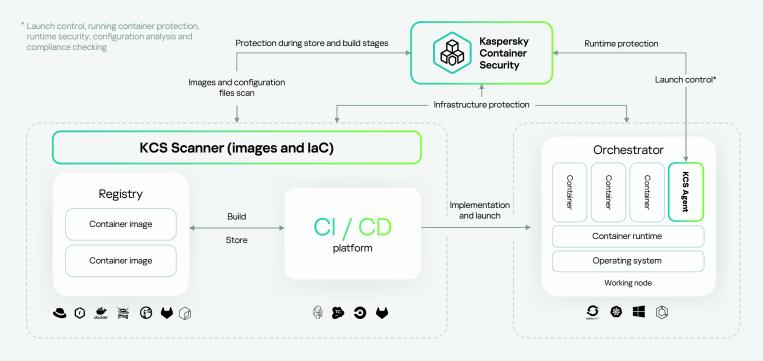
Kaspersky Container Security (KCS) enables protection at every stage of app design and operation. It consists of three components: KCS Agent, KCS Scanner and KCS Control Server.
