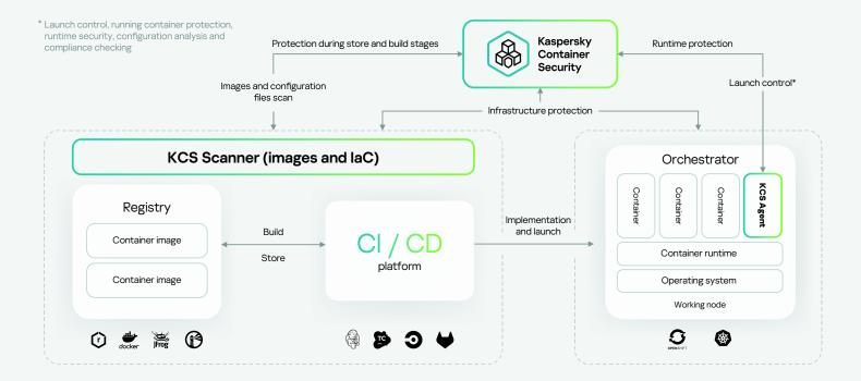
Kaspersky Container Security (KCS) enables protection at every stage of app design and operation. It consists of three components: KCS Agent, KCS Scanner and KCS Control Server.
